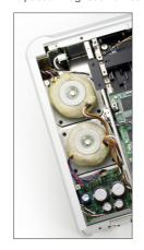
The K-03 features two large-capacity toroidal transformers, including one specifically for the built-in dual mono D/A converters and the audio circuits, and the other for driving the digital circuit and mechanism. This design provides dedicated power supply capability to all circuit blocks without interference.
